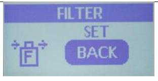
As soon as Menu is pressed after selecting the fourth digit, you return to this screen, If you press BACK no new value is selected and the current value is not reset. If the current value and the selected value are the same the menu does not show the BACK option. If, for example, you reset the value to 1525 Gal (or L), exit the filter menu, then come right back in, you will not see a BACK option since the set value and the current value are still the same.
