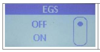
Use the Up arrow or the Down arrow buttons, move the Dot to ON or OFF, then press the Menu button to lock in that option and return to Menu screen #2.
