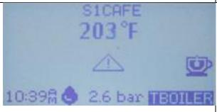
After an alarm has been active for one minute the descriptive text goes away and is replaced by the alarm icon in the middle of the screen. If you weren't looking at the screen when the above message was displayed and you only see the icon in this photo, you can go to a screen (see paragraph 6.2) and redisplay the text for this alarm as well as for any other alarms that are currently active.
