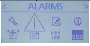
With the large Alarm icon displayed and the word ALARMS showing at the top of the screen, press the Menu button.
