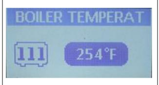
Use the up or down arrows to increase or decrease the indicated temperature until the desired steam temperature is showing. Note that unlike the coffee temperature, you are aiming for a temperature here that produces the desired steam boiler pressure as indicated by the manometer on the front panel behind the group.
