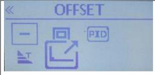
With the large Square and Diagonal Arrow icon displayed and the word Offset showing at the top of the screen, press the Menu button.
