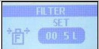
At this point the 2<sup>nd</sup> digit from the right is blinking. Use the up or down arrow buttons to set this to your desired number between 0-9. Then press the Menu button to lock in the value of this digit.
