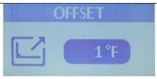
Use the Up and Down arrows to scroll to your desired value, then press the Menu button to lock in the value and return to Menu screen #4.
