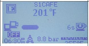
This display shows what the screen looks like during a shot. The two cup icon on the left indicates that the 2 cup button was pushed. Alternately, the one cup icon would display. The bar shows the shot time relative to the total programmed shot time and the "6s" indicates that we are 6 seconds into the shot. The final time value at the end of the shot remains for 10 seconds or until the next shot is started, whichever comes first.
