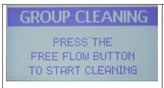
Press the Continuous Flow button (the one between the One-Cup and Two-Cup buttons) to begin the cleaning operation. It continuously cycles 5sec On / 5sec Off.
