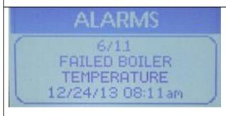
This and the next three screens show an examples of four alarm history screens from this Dream machine. Note that this is alarm 6 of 11. You use the Up and Down arrow keys to scroll back and forth through the list. Note that details of the alarm as well as the date and time it occurred are displayed.
