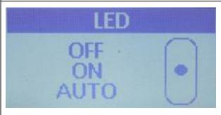
Use the Up and Down Arrows to select OFF, ON, or AUTO, then press the Menu button to lock in the value and return to Menu screen #2.
