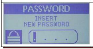
Next use the Up and Down arrow keys to scroll through the choices for the 1<sup>st</sup> character. Only the numbers 0-9 are available and only four characters are used so this is really a PIN number more so than a password.
