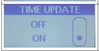
Use the Up or Down arrows to select either OFF or ON and then press the Menu key to lock in the selected value. If OFF is selected there will be no automatic Daylight Savings time adjustment. If On is selected you are taken to the next screen to pick your desired option.
