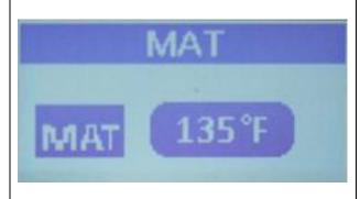
If you just couldn't help yourself on the previous screen and selected ON before pressing the Menu key, you will see this screen. You can use the up or down arrows to select a desired milk temperature, then press Menu to lock it in and exit to the main Profile menu. At the moment the only impact of this setting is to cause an alarm
