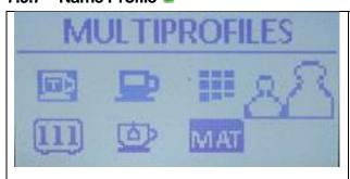
Depending on where you are in the profile menus, press the Up or Down arrow to highlight the Profiles icon and display that text on the top of the screen. Then press the Menu button to enter the PROFILES programming screen.
