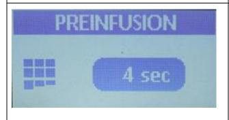
On this screen you select the number of seconds you desire for preinfusion. The value selected here indicates the number of seconds during the shot that the water is turned on running into the PF at street pressure before the pump is turned on. The amount of water programmed when you set the coffee doses is not impacted by the value used here since the total shot volume is measure by impeller turns any time the water is flowing.
