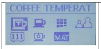
Starting from the last menu in the previous section, press the Down arrow to highlight the Coffee Temperature icon and display COFFEE TEMPERAT on the top of the screen. Then press the Menu button to enter the Coffee temperature (group boiler) programming screen.
