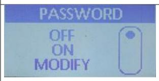
Use the Up or Down Arrows to select the desired password mode. If you do not want the configuration menu to be password protected set this to OFF. If you want the password protection feature, turn this setting ON to use the current password. If either of these options is selected, pressing the Menu key locks in that value and returns you to Menu screen #3. Selecting Modify and then pressing Menu takes you to the next screen.
