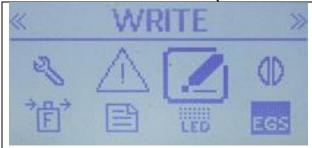
With the large Write icon displayed and the word Write showing at the top of the screen, press the Menu button.
