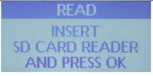
With the SD card that came with your machine inserted into the reader, plug the ribbon cable connector in to the port to the right of the pressure gauge. Then press the Menu (OK) button to start the backup of your machine
