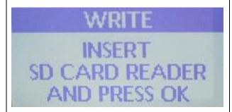
With the SD card that came with your machine inserted into the reader, plug the ribbon cable connector in to the port to the right of the pressure gauge. Then press the Menu (OK) button to start the restoration of your previously backed up machine settings.
