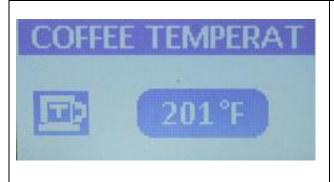
Use the up or down arrows to increase or decrease the indicated temperature until the desired espresso temperature is showing.
