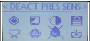
With the large "Drop with and X through it " icon displayed and the word DEACT PRES SENS showing at the top of the screen, press the Menu button.
