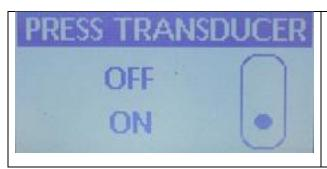
Use the Up or Down arrow keys to select either OFF or ON, then press the Menu key to lock in the selected value.
