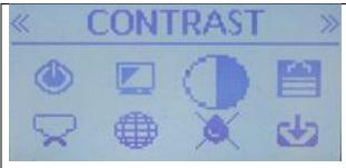
With the large  $\frac{1}{2}$  clear/  $\frac{1}{2}$  dark circle icon displayed and the word CONTRAST showing at the top of the screen, press the Menu button.
