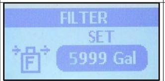
Caveat: The above process will let you set these four digits as high as 5999 Gal or L. However, the highest settable value is 5000. Therefore, if you set the value from 5001 to 5999, when the Menu button is pressed the value 5000 is locked in.
