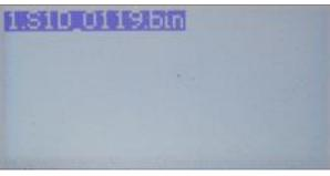
Next the Dream display lists all .bin files it has found on the card. Use the Up and Down arrows if you have multiple .bin files in order to highlight the correct one, then press the Menu button.
