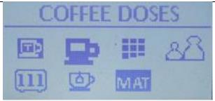
Depending on where you are in the profile menus. press the Up or Down arrow to highlight the Coffee Doses icon and display that text on the top of the screen. Then press the Menu button to enter the coffee doses (water volume) programming screen.
