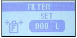
From the previous screen, pressing the Menu button brings you to this filter set screen with the right-most (LSB) digit blinking. Use the up or down arrow buttons to set this to your desired number between 0-9. Then press the Menu button to lock in the value of this digit.
