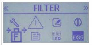
With the large filter icon is displayed and the word FILTER showing at the top of the screen, press the Menu button.
