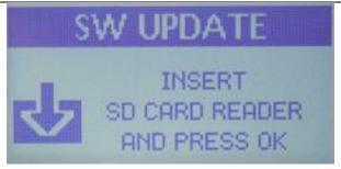
Plug in the SD Card reader with the SD Card containing the firmware update file inserted. Since files with an extension of .bin are usually blocked from FTP downloads or e-mail attachments, new firmware versions are usually zipped. You will need to unzip the file and use a PC connected card reader (this one can't be used) so that you can unzip the .bin file and copy it to this SD Card. When ready press the Menu/OK button.
