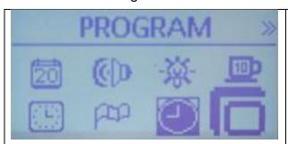
Starting with the Program icon on menu Screen 1 highlighted, press the Down arrow to bring up Menu screen #2.
