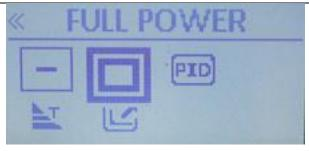
With the large Double Square icon displayed and the word FULL POWER showing at the top of the screen, press the Menu button.
